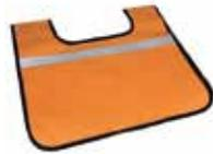
**Wire Rope Dampener:** The purpose of this accessory is to reduce the risk of injury due to recoil in the event of a winch line or recovery strap failure (The whip effect). It has the shape of a blanket with pockets to be filled with weights like sand or stones. Once loaded should be folded around the wire rope before pulling.
